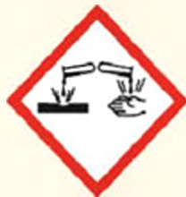
Corrosif (Ça ronge)
